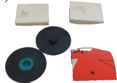
Figure 5 a) Samples of portion of helmet. b) Detail of one sample containing the O-Damp system
