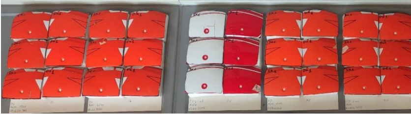
Figure 5 a) Samples of portion of helmet. b) Detail of one sample containing the O-Damp system
