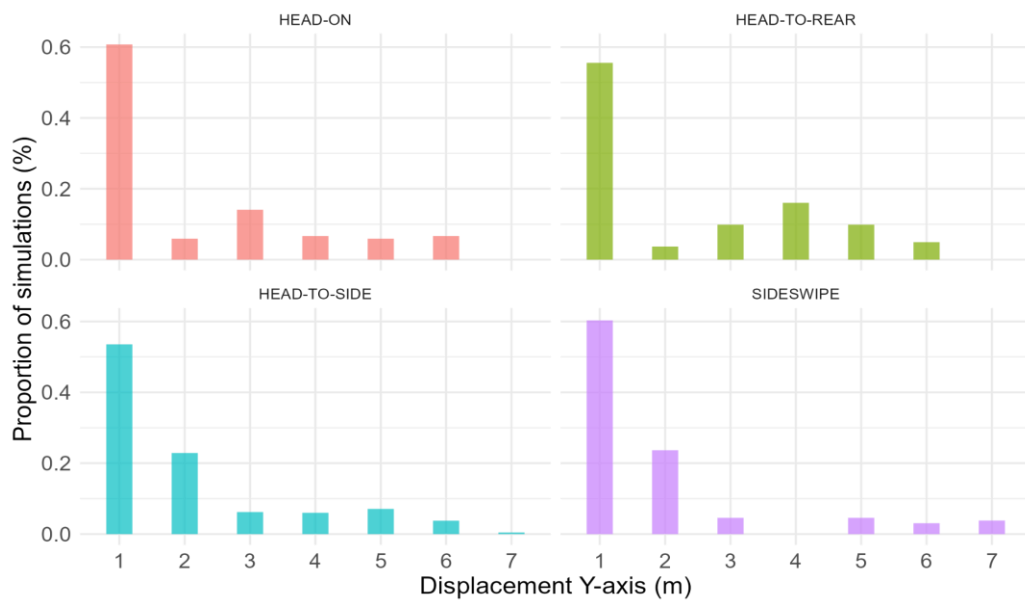
Figure 6 - Lateral displacement of PTW after MAES intervention clustered for crash configuration
