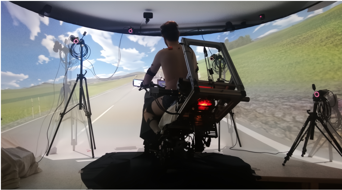
Figure 1: Image taken during one of the recorded runs. Four of the seven Miqus M3 cameras are visible here.
