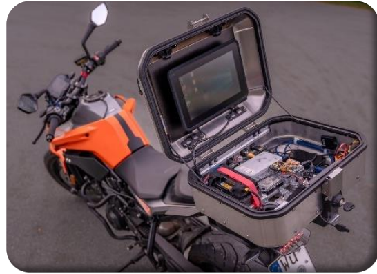
Figure 5: Target route of the naturalistic riding study & measurement motorcycle (KTM 790 Duke)
