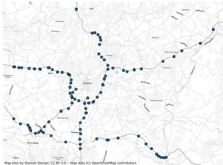
Figure 9: Detector locations on the Luxembourg highway network
