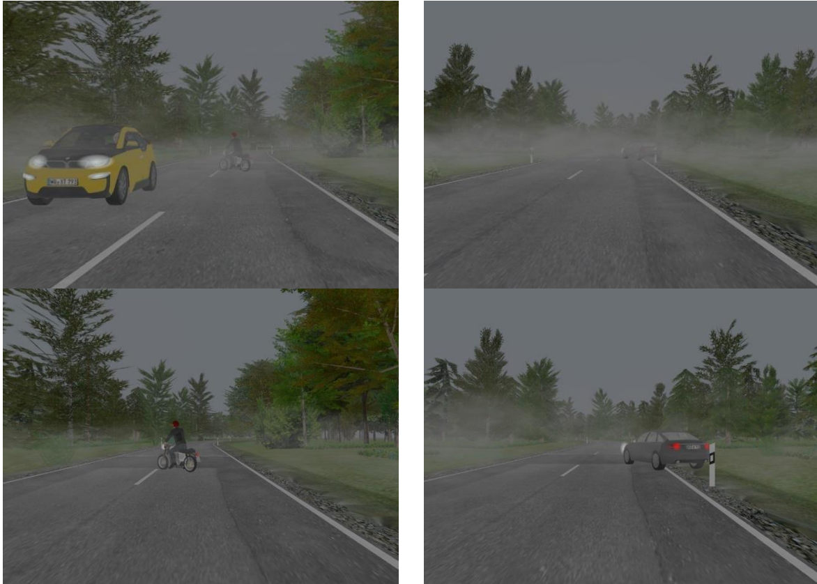
Figure 2: Local Hazard Warnings: PTW (left) and passenger car (right) test scenario with obscured obstacles due to ground fog (upper row) and recognizable obstacles when approaching the test scenarios (lower row).
