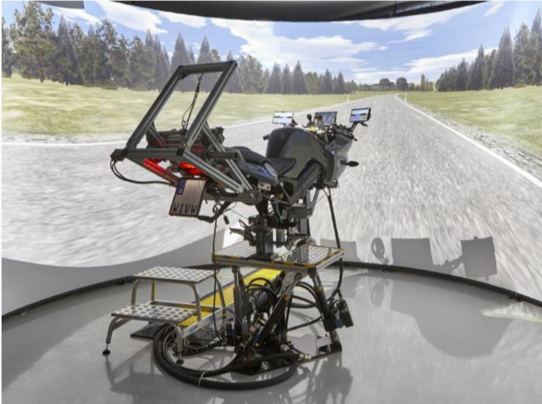
Figure 4: Dynamic motorcycle simulator
