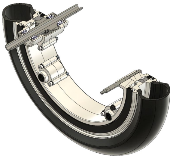
Figure 10: Traction-X® drivetrain suspension cross-section
