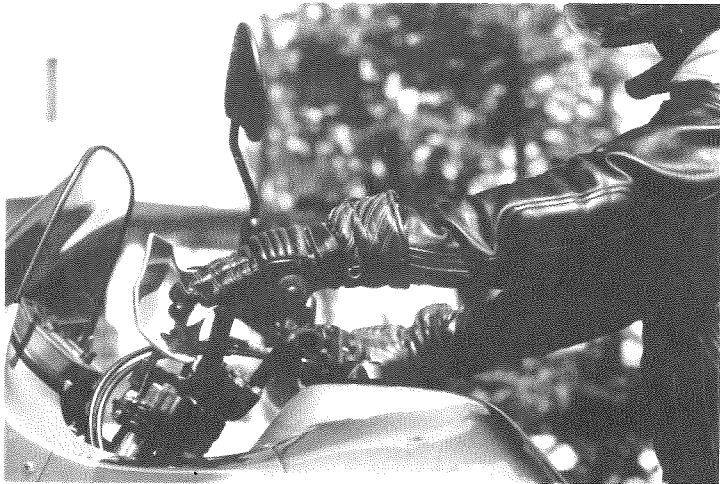
Pict. 5: Optimum lever arrangement: a straight line along the lower arm / back of the hand / fingers
