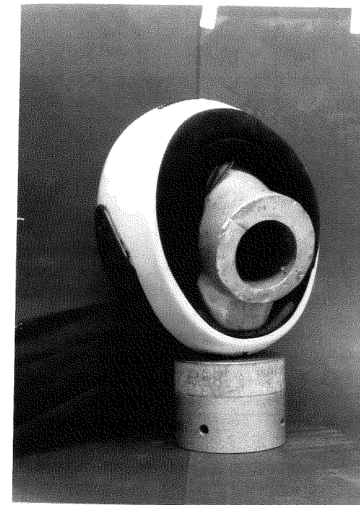
Fig. 2: Positioning of the headform for the chin section test (ECE-R22 - aluminium head for shock absorption testing)
