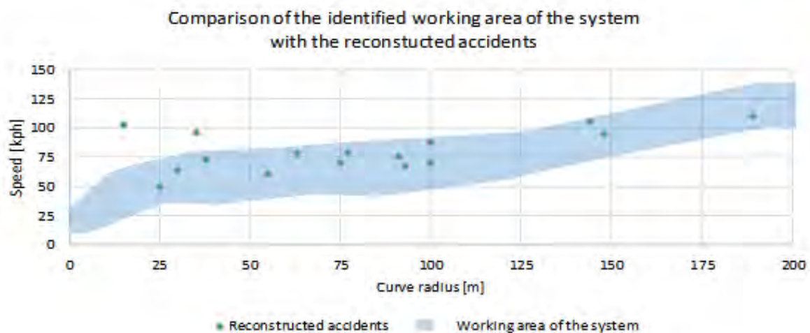
Fig. 10: Comparison of the identified working area of the system with the accidents parameters for accidents in a bend. Note that only the accidents in a bend with a radius minor than 200 meters (94 % of the considered accidents) are displayed.
