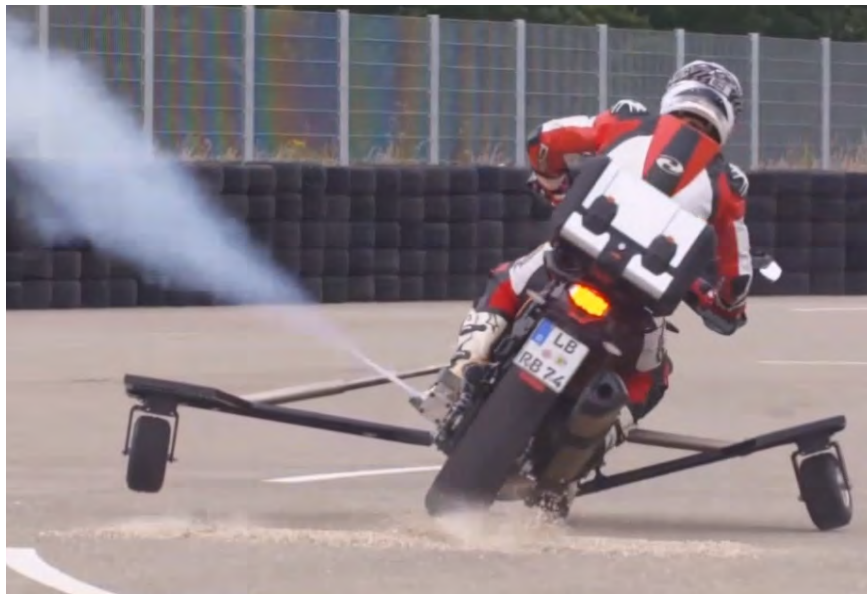
Fig. 6.4: Riding test with an actuator intervention on the rear
