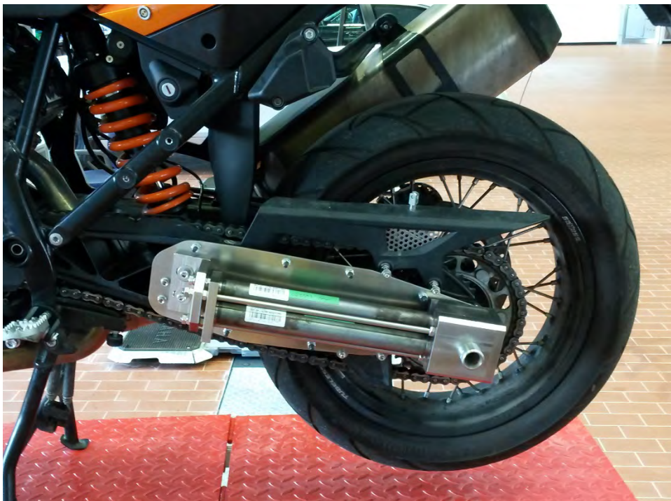
Fig. 6.2: Repulsion actuator with three cold gas generators (CGG) on the rear arm swing
