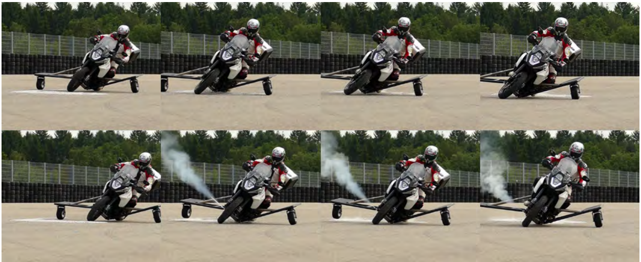
Fig. 6.6: Testing of the repulsion actuator mounted on the front of the sprung mass. Upper sequence: actuator deactivated, lower sequence: actuator active.
