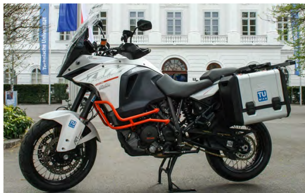
Fig. 1: KTM 1290 Super Adventure equipped and instrumented as a Motorcycle Probe Vehicle (MoProVe) .
