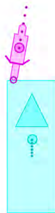
Fig. 3: Example vehicle impact geometry based on the coded impact locations and the relative heading angle (MAIDS case MAF01283).
