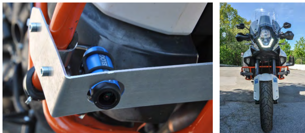
Fig. 4 a) HD-camera system mounted on MoProVe; (b) Mounting of both cameras.
