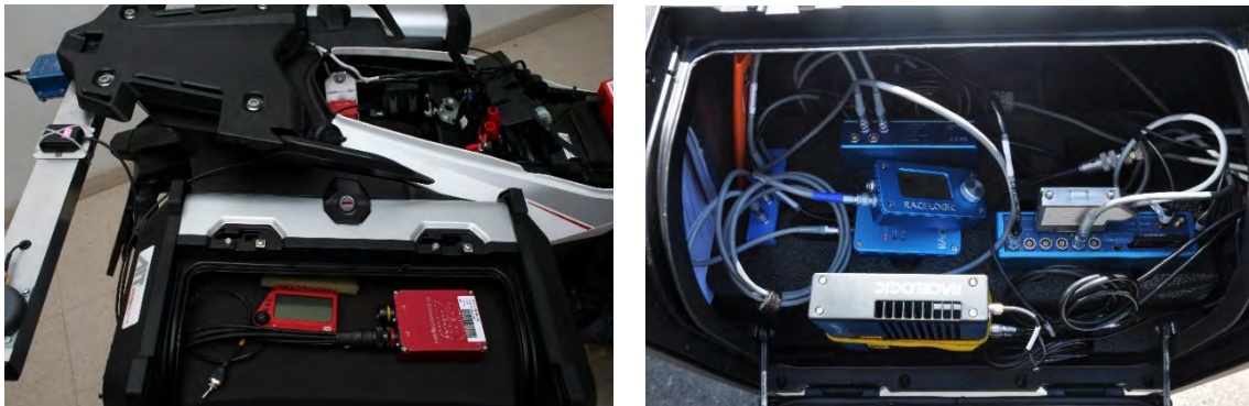
Fig. 6: a) Side case on the right hand side, containing System R, 2D data logger and display; (b) Side case on the left hand side, containing System B, logger VB3iSL, connectors and accessories.
