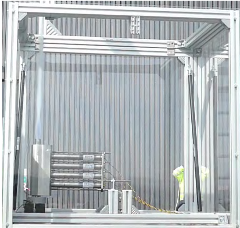
Fig. 6.3: Test rig for the force measurement of the actuator prototype
