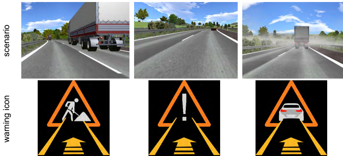
Fig. 3: Scenarios and corresponding warning icons for the different C-ITS applications (from left to right: Roadworks Information, Road Hazard Information, Forward Collision Information).
