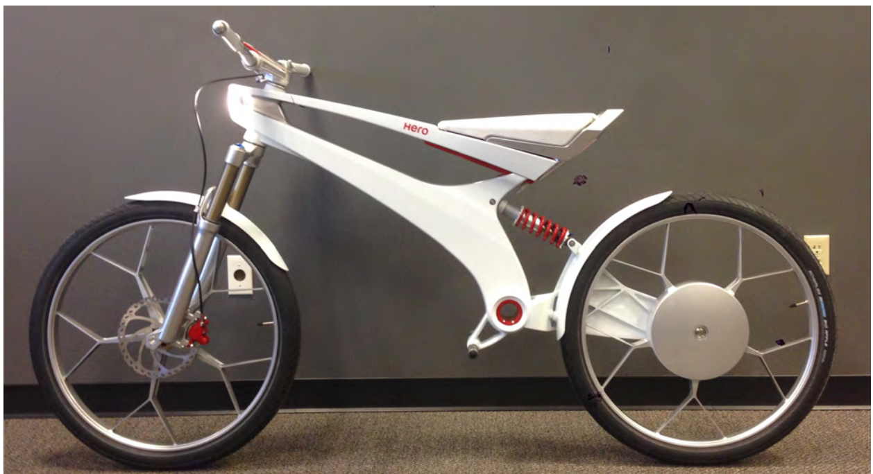
Fig. 7: Early styling prototype of proposed EBR electric L1e vehicle. Battery was encompassed in the seat, which was removable. A 4kW hub motor of advanced design provided power.
