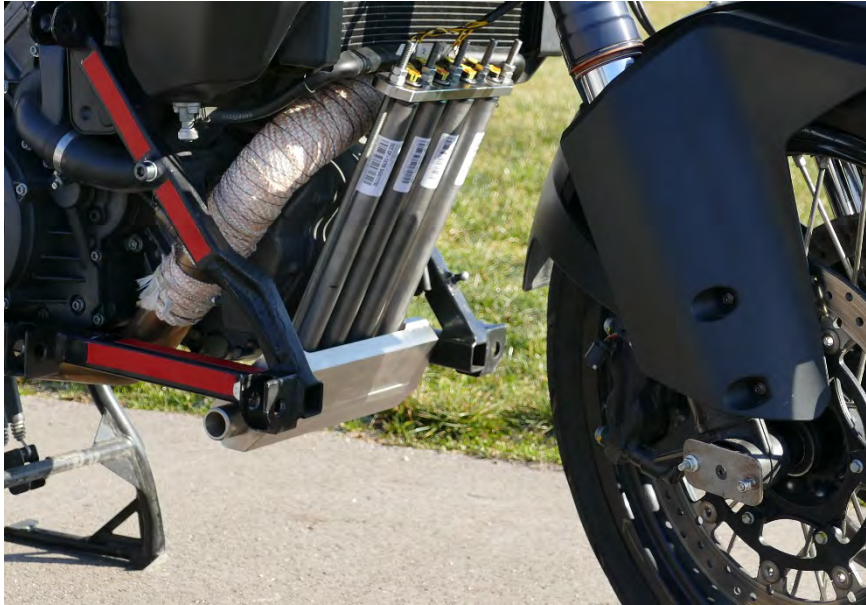
Fig. 6.1: Repulsion actuator with four cold gas generators on the sprung mass
