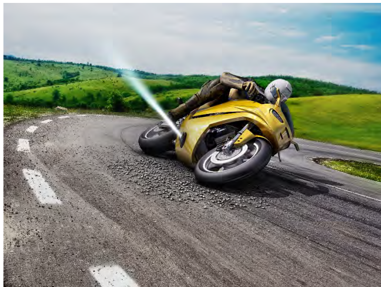
Fig. 1.1: New actuator concept: repulsion forces offered by fast escaping gas
