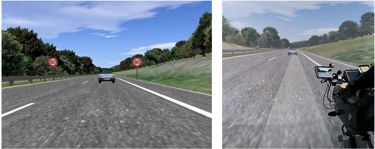
Figure 1. Lead vehicle on the highway test course (left). Grey enhanced reality strip indicating the proper distance to the lead vehicle ahead (right).
