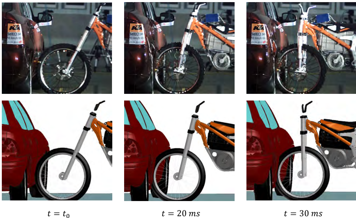
Figure 11. Different instant of the simulation of crash configuration number 1 and of the full-scale crash test.
