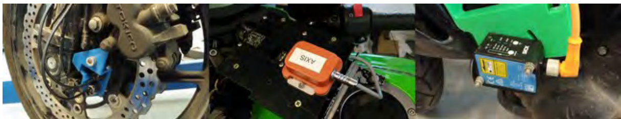
Picture 1. some sensors on the Kawasaki: wheel, the two IMUs, a laser
