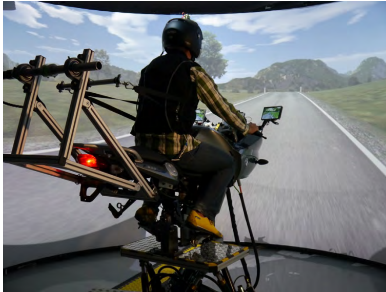
Figure 2. DESMORI motorcycle riding simulator at WIVW.
