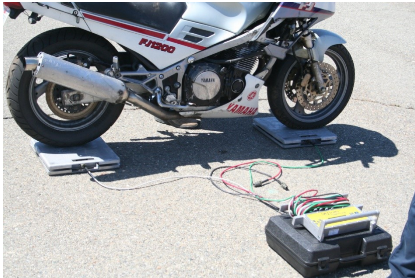
Figure 3. Yamaha FJ1200 being weighed using digital scales.
