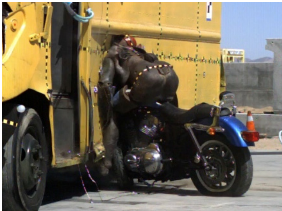
Figure 2. Interaction of the motorcycle, rider and crash partner at maximum crush.
