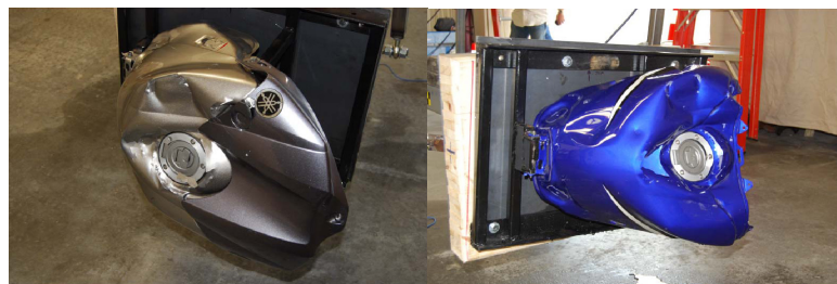
Figure 9. Test Tank Damage for Both Tests. Grey Tank was tested at 12.8 kph. Blue tank was tested at 16 kph.
