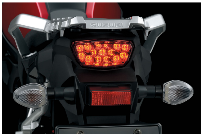
Suzuki stop and tail light uses LED technology for greater response and improved reliability.
