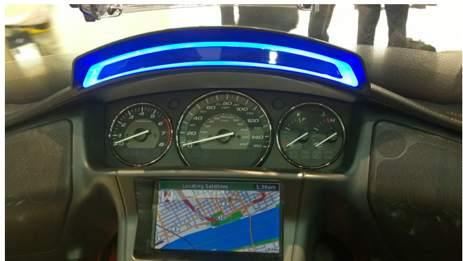
The HMI developed by Honda provides a visual and an audible warning in safety critical situations. The visual element is located close to the rider's line-of-sight and uses changes in color and intensity to communicate the nature of the threat.
