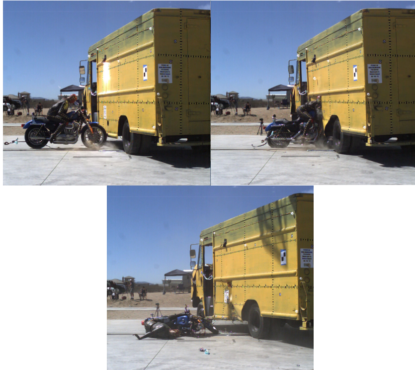
Figure 1. Interaction of the motorcycle, rider and crash partner at initial contact, maximum crush and at rest.
