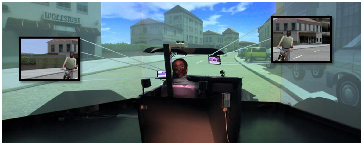
Figure 4. Car driving simulator with highlighted rear-view and wing mirror.
