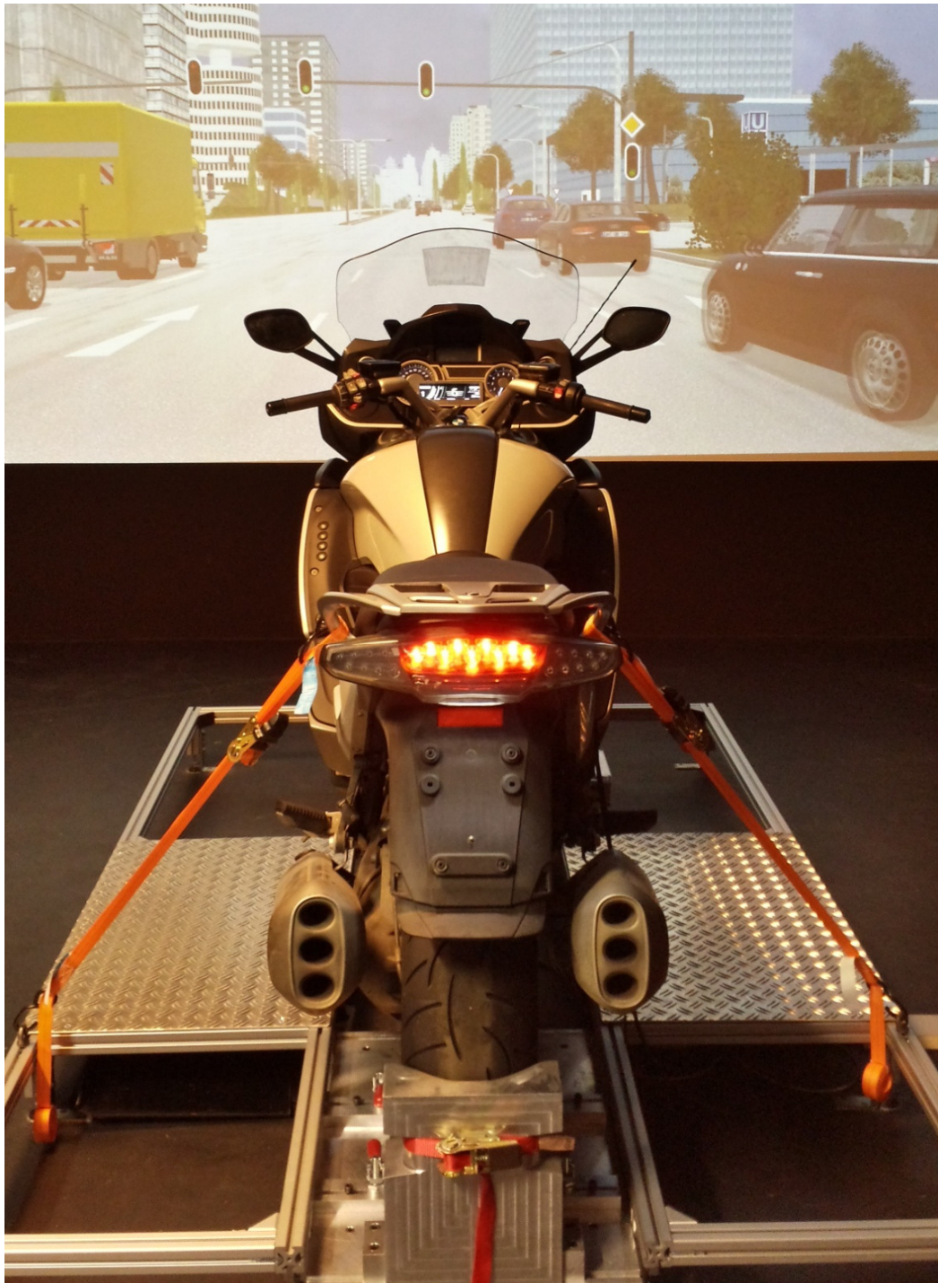
Picture 3. Simulator mockup built on a BMW K1600 GT motorcycle
