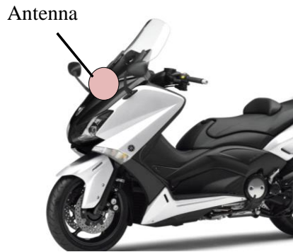
Figure 2. placement of antenna
