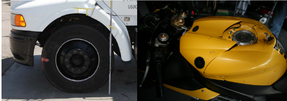
Figure 7. Impacted truck and motorcycle tank damage.
