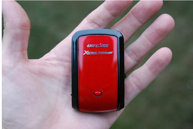
Figure 1. QSTARZ BT-Q1000eX GPS lap timer / data logger.
