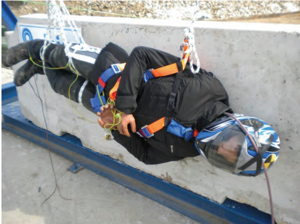
Figure 35. Hybrid III dummy after the shoulder impact with airbag device (test n. 18).
