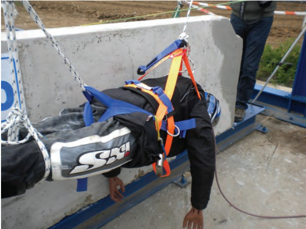
Figure 34. Hybrid III dummy after the shoulder impact with airbag device (test n. 9).
