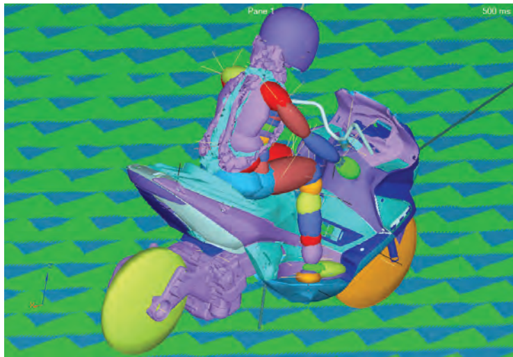
Figure 5. TNO MADYMO. Hybrid III dummy model wearing the airbag jacket in riding attitude after the dressing simulations.
