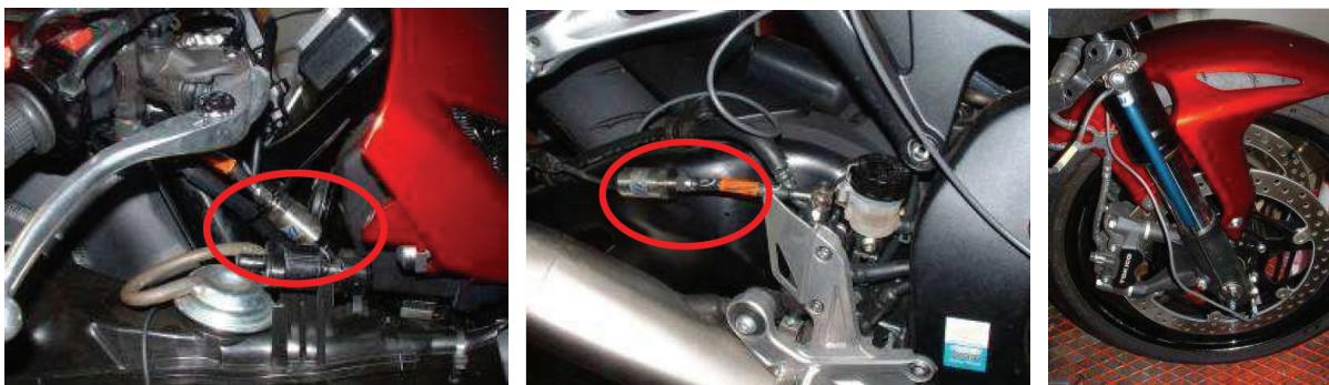
Figure 1: Sensors on CBR1000RR at TRL
