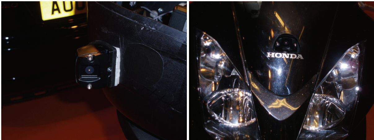
Figure 3: Side and front camera on CBF1000 at INRETS
