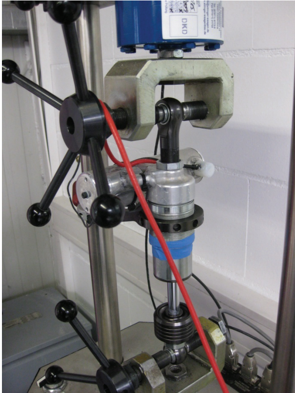
figure 7: ER motorcycle damper with external valve (in the piggyback) on a servohydraulic test bench
