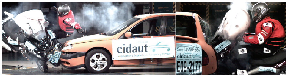
Figure 14 - Crash tests in 114 and 413 configurations with airjacket + frontal airbag
