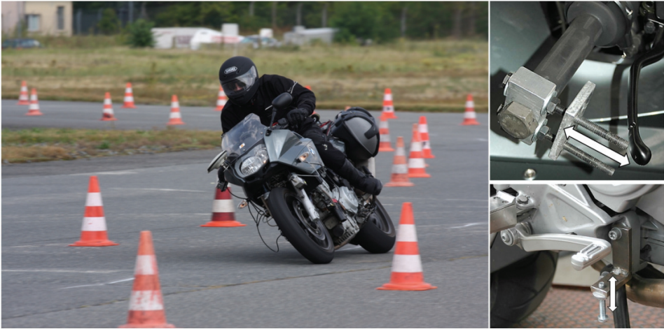
Figure 7: BMW F800S test bike equipped with measurement devices and manually adjustable brake lever stops during corner braking experiments.
