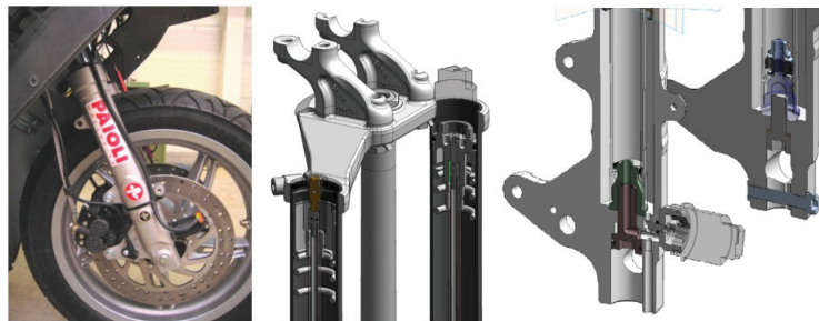
Figure 13: Semi-active front fork installed on the Malaguti
