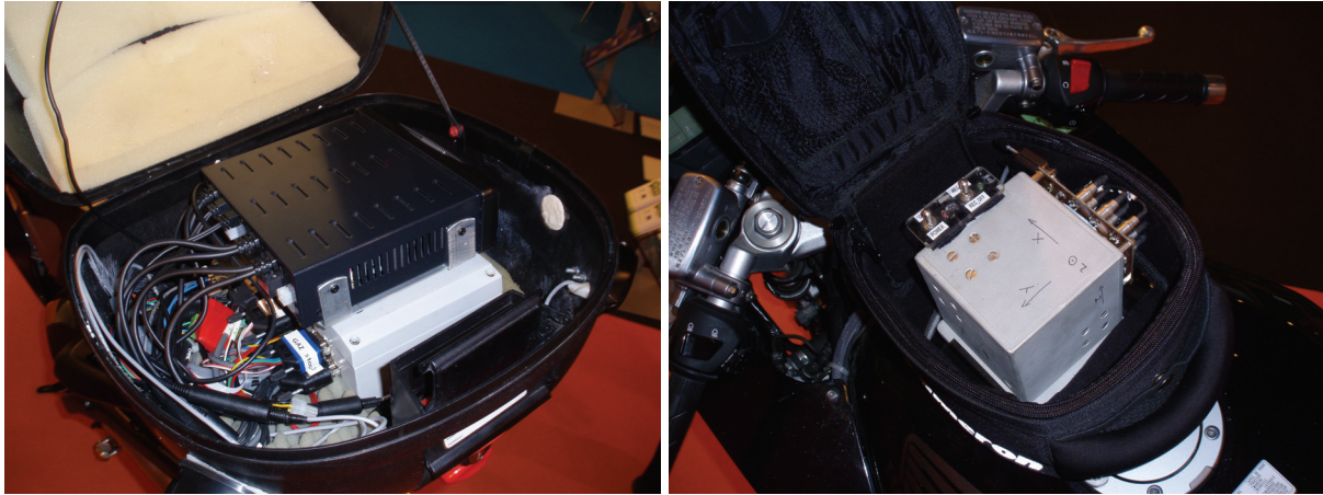
Figure 2: Data logger in top Case and tank pack on CBF1000 at INRETS
