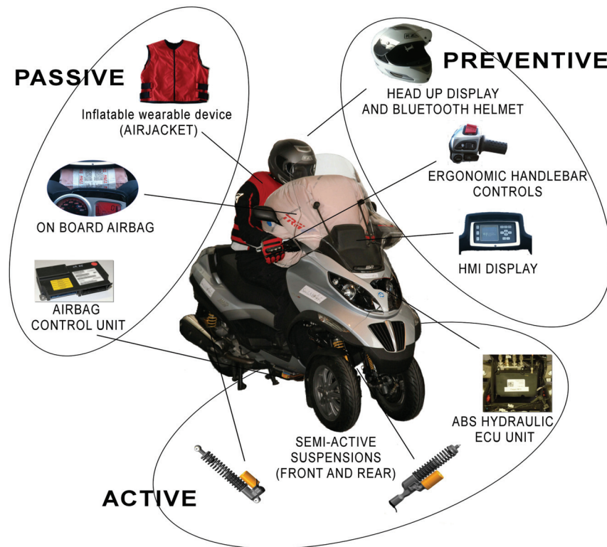
Figure 4 – SIM integrated prototype with all safety features
