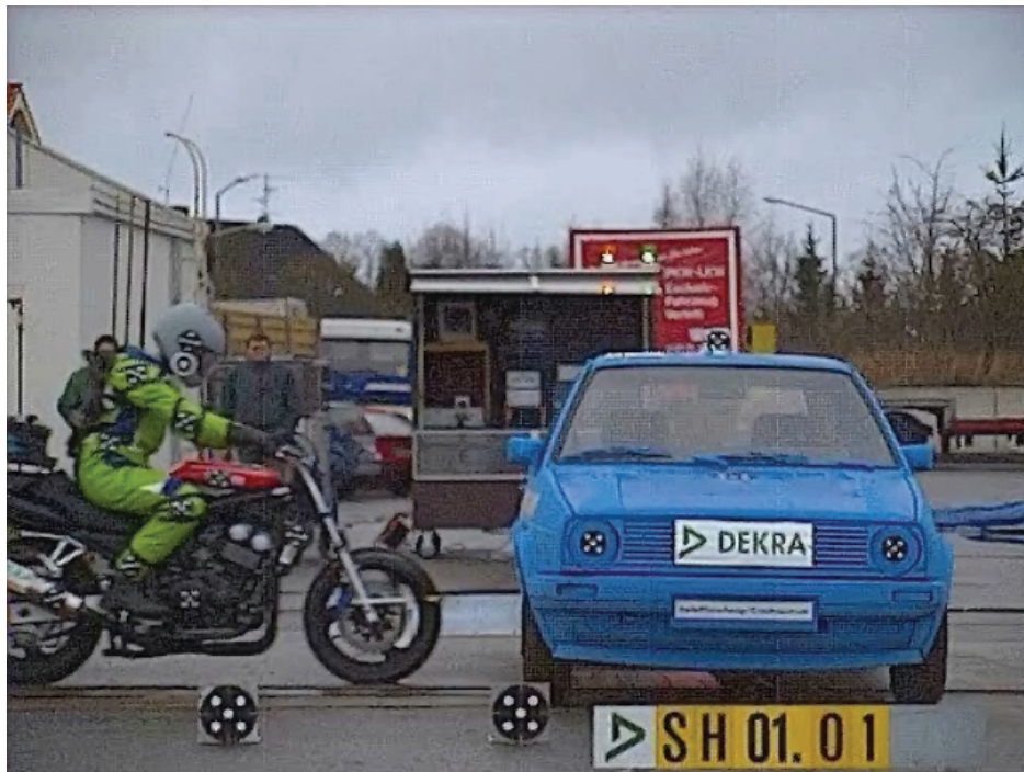
Figure 3: Crash test (performed by DEKRA) used for validation of the numerical models
