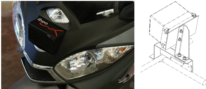
Figure 5: Integration of the Ibeo Lux Laserscanner
