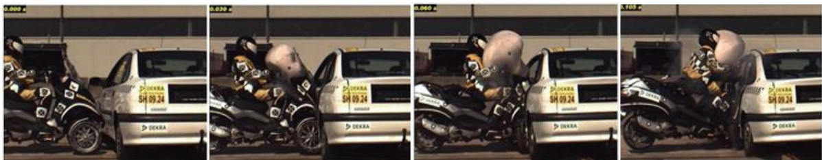
Figure 13 – Pictures sequence of full-scale crash test in 413 configuration with airbag
