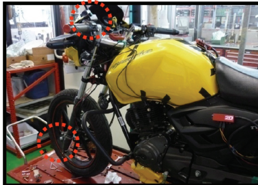
Figure 19: Anti-dive suspension on the TVS motorcycle
