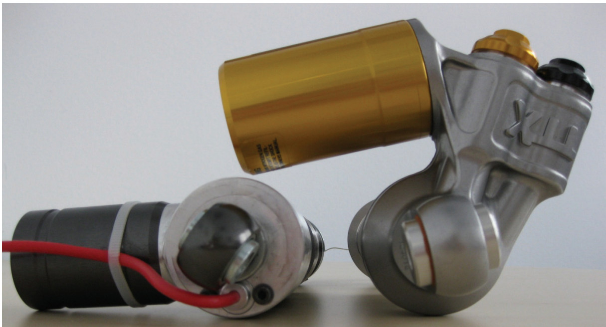
figure 9: comparison of eRRide motorcycle damper with internal ER valve (left) and conventional adjustable retrofit damper (right) regarding size
