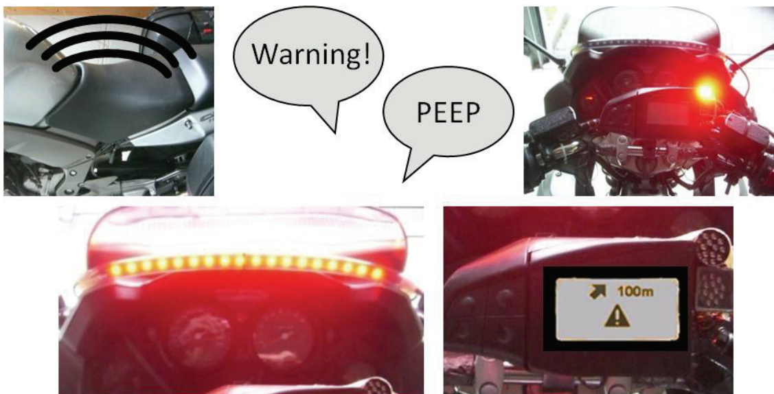
Figure 3: Warning Elements: Haptic Saddle, Auditory Warning, Warning Flashes, LED-Band, Display
