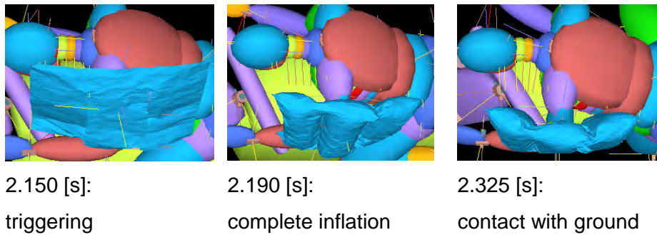
Figure 17: Inflation sequence of a simulated 12 liter airbag system
