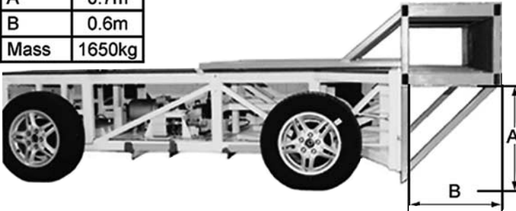
Figure 19 Opposing trolley used in under-ride collision tests
