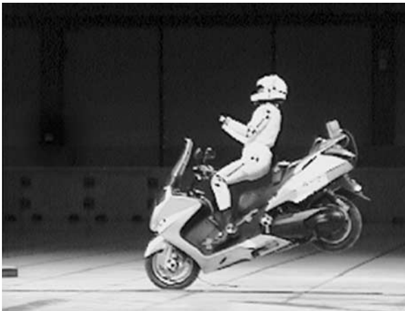
Figure 2 Motorcycle and dummy in simulated curb ride over test
