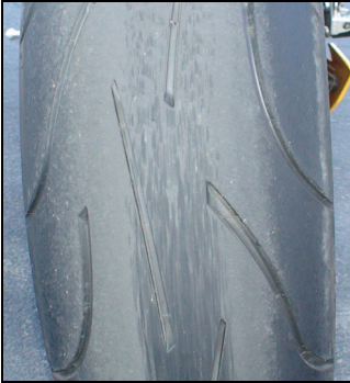
Figure 11a. Feathered onset of abrasion.
