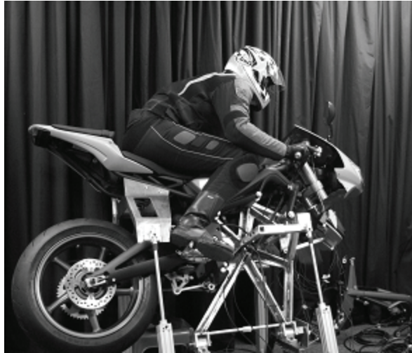
Figure 1: MotorcycleSim with a rider leaning into a corner
