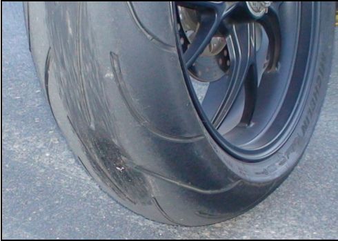
Figure 11b. Heavy end of abrasion.
