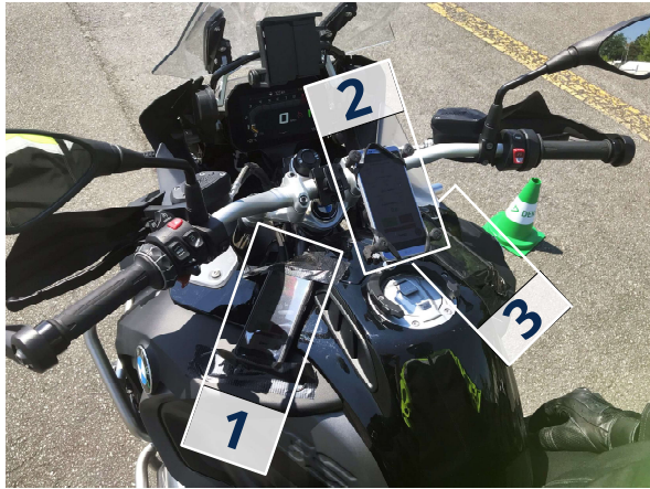
Figure 17. Three smartphones mounted on the test motorcycle in different orientations
