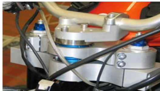
Figure 2: Steering torque measurement with torque measurement shaft
