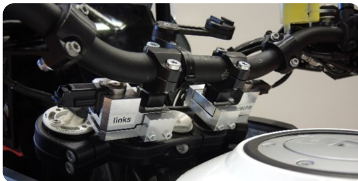
Figure 7: Steering torque measurement setup
