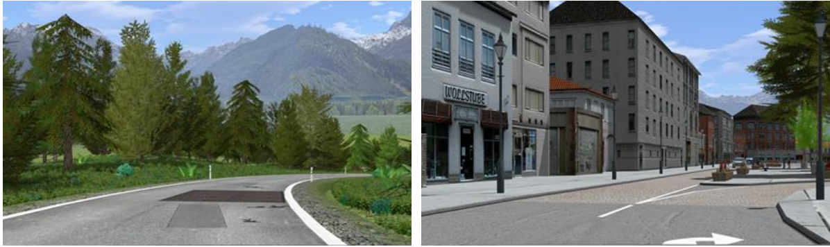
Figure 5: Exemplary test scenarios. Rural road (left) and urban road (right) with changing road surface (low friction ahead).
