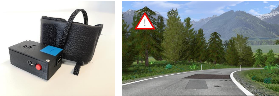
Figure 3: Haptic device (left) containing a bracelet and the controller. Simulated Head-Up Display warning icon (right).
